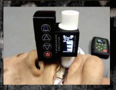
Designed to be used as a mainstream carbon dioxide monitor that can be connected in-line with a mask or tube.
