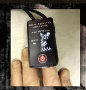
The ITTS Pulse Oximeter simulator utilizes the widely used finger-style probe for monitoring blood oxygen saturation.
