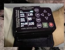
Designed to replicate a portable NIBP monitor, this simulator allows medical responders to gather vital signs without instructor intervention. Onboard controls allow various modes of operation. Display includes systolic & diastolic pressures (mmHg) and heart rate.
