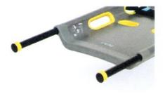
Handles are retractable with a built-in stopper. Handles are locked in position by turning the handle either way.
